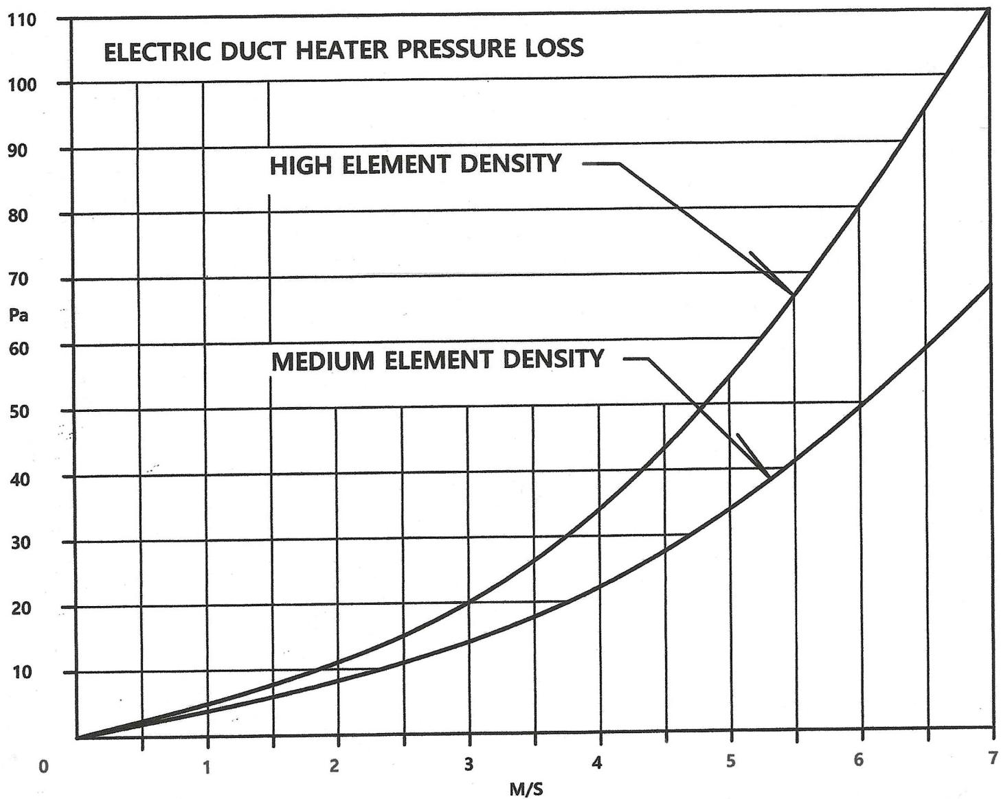
**NB: ELECTRIC HEATERS WILL INCREASE SURFACE TEMPERATURE AT LOW VELOCITIES. MIN 1.5 M/S**
