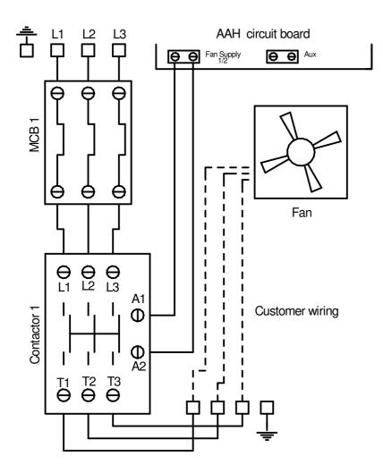
AAH 3 phase fan module Wiring diagram for three phase fans Customers are to provide an additional supply for the fan complete with isolation and protection.
